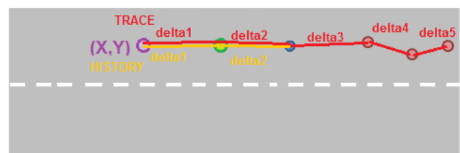
figure 7. Coding principles for a linear event from the vehicle
